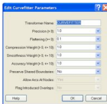
Figure 1: Dialog box for setting Curvefitter Parameters. (Click for larger image)
