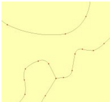
Figure 5 c) optimized linework after Curvefitter; note that a vertex at an intersection was maintained during optimization. (Click for larger image)
